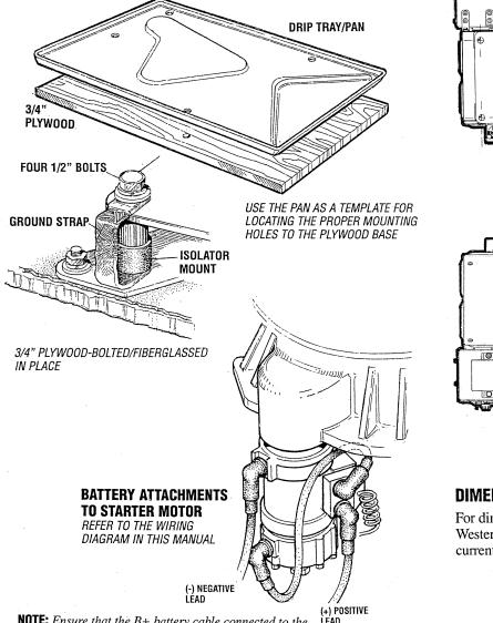
**NOTE:** Ensure that the B+ battery cable connected to the remote mounted starter solenoid is properly supported to prevent unwanted stress on the solenoid.
