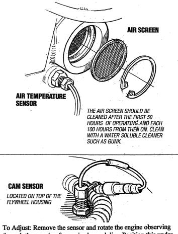
through the opening for a raised round disc. Position this under the opening. Thread the sensor in until it touches the disc, then back it out  $\frac{1}{4} - \frac{1}{2}$  turn and lock it in position.
