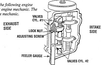
7. Adjust the intake and exhaust valve clearance for cylinder #2 using the same sequence.
