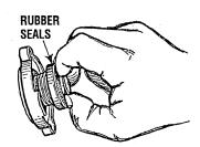
**NOTE:** Periodically check the condition of the pressure cap. Ensure that the upper and lower rubber seals are in good condition and check that the vacuum valve opens and closes tightly. Carry a spare cap.
