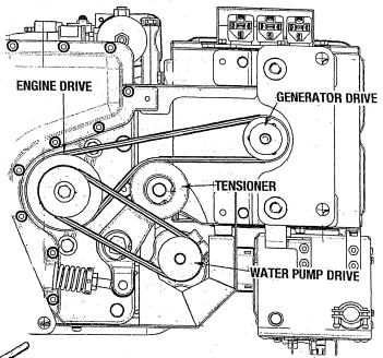
The Idler Arm/Spring should not BOUNCE more than 1/8-3/16 of an inch during normal, steady state operation. Excessive Idler bounce can be caused by insufficient drive belt tension. Operating with an insufficient drive belt tension and Idler bounce can result in premature drive belt wear and resulting failure. This applies to both older and current models.
