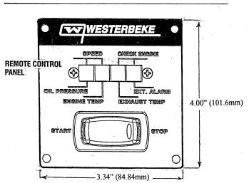
**REMOTE PANEL** (with Fault LEDs) An optional remote panel and plug-in extension harness are available that allows for remote operation of the generator. The Start/Stop sequence is identical. Once installed, the engine can be operated by either panel.
